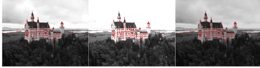
Figure 4: Harris interest point detector applied to original image [686 corners detected], original image with all pixel values scaled by 1.5 [590 corners detected] and original image with all pixel values scaled by 0.85 [683 corners detected]
